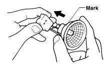
5 Insert the new Projection Lamp all the way into the Lamp Holder.
